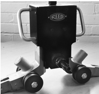
2. Tighten Long Arbor onto motor unit
