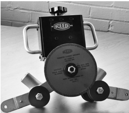
5. Slide on 97066 Flanged Washer and then tighten 97543 Flexloc Nut
