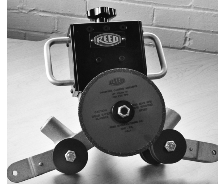
5. Slide on 97066 Flanged Washer and then tighten 97543 Flexloc Nut
