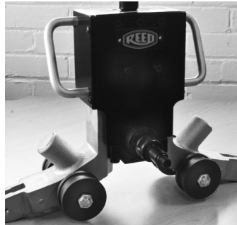
2. Tighten Long Arbor onto motor unit
